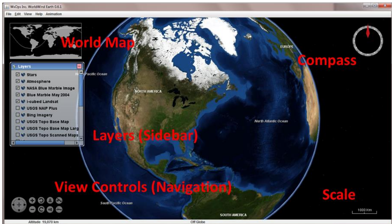
Figure 2 – Configuration of controls on the WorldWindUI Canvas when started up as WxOps WorldWind Earth (WWE).
